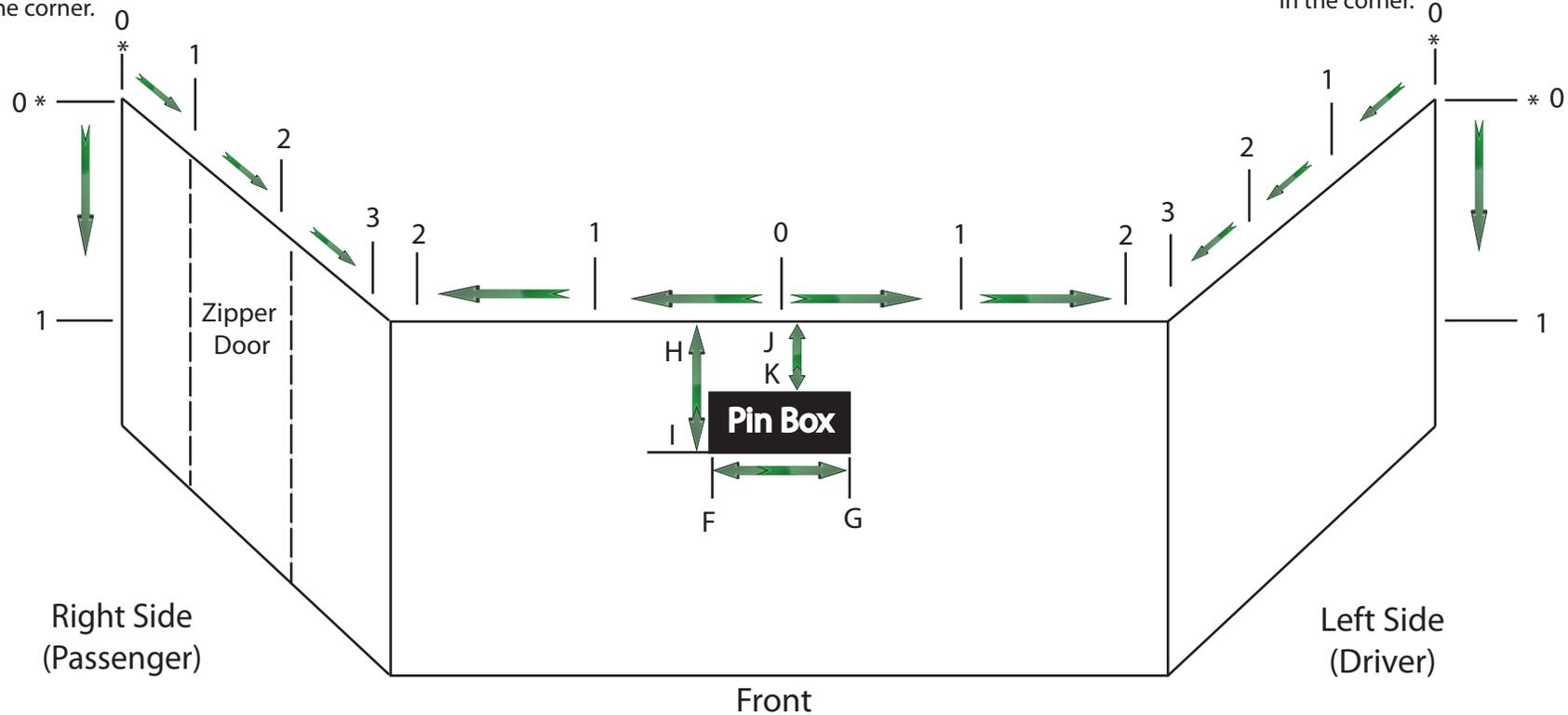
Please start at Zero and follow the direction of the arrows when measuring for the Eyelet placement. In most installations it is probably best to mark your Zero points on the sides of the trailer. Visualize the installation and how you will install it and that will help to reduce mistakes in measuring. Please keep in mind, we can't see the 5th wheel and not all 5th wheels are the same. It is up to you to provide us with accurate measurements.
